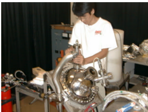
Figure 1. An IECF device, with a spherical hollow cathode in a spherical vacuum chamber as an anode
